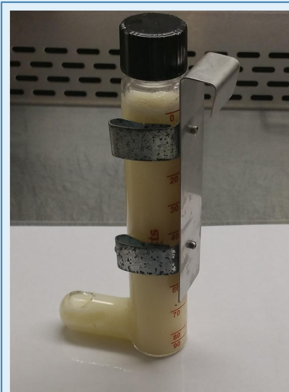
Image (left) shows a J-feeder used to administer diet to all animals through a week of pre-treatment and until GD20.
